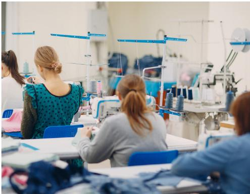
For example, some businesses choose to use a cost-effective batch SFC solution to manage and track sub-assembly work, such as making collars and cuffs. Real-time visibility to this production stage may not be as meaningful as visibility to final assembly and finishing. Daily updates on sub-assembly work often are sufficient.
